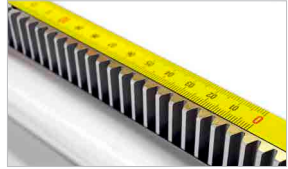
Bar with millimetre scale to visualize the cutting size of the rolls
