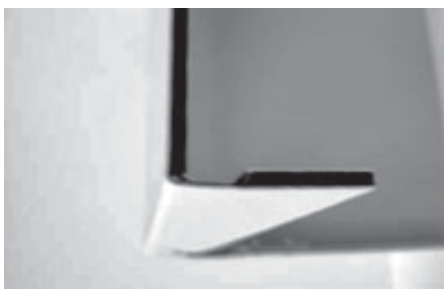
Distorted Flat Rout Folded 90°
